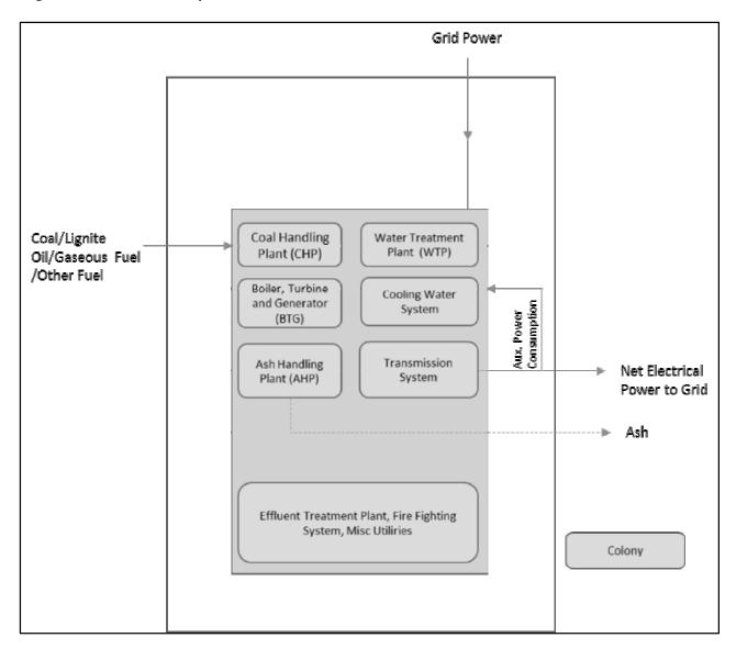
The colony does not form a part of the plant boundary and hence it is kept outside. In the figure above. The DC shall submit a latest Plot Plan of the station indicating all the systems/ sub-systems.
